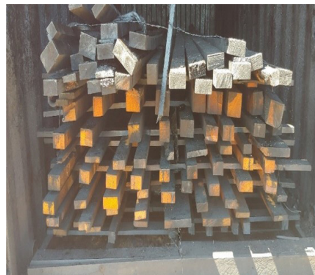
Photo of rough sawn logs in drying kiln.
