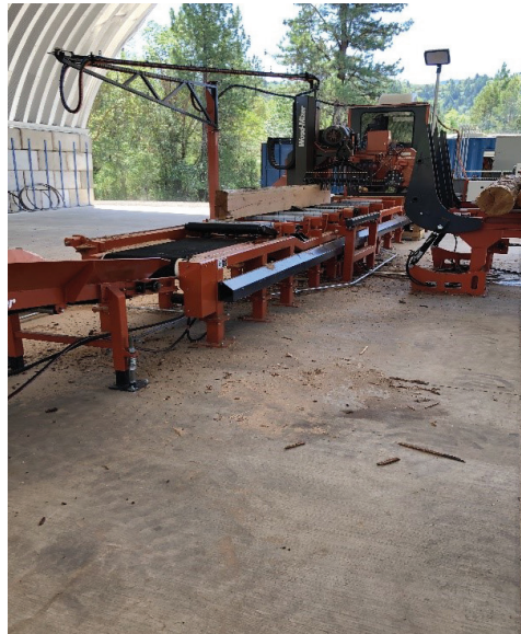
left: Photo of Cow Creek Portable Sawmill Processing Fire Salvage Logs.
